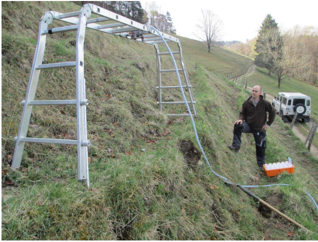
Figure 5. The adjustable aluminium frame supporting the rainfall simulator. Such a configuration allows the simulator to be firmly supported and level, even on challenging terrain such as a well-developed terracette system on a steep slope.
