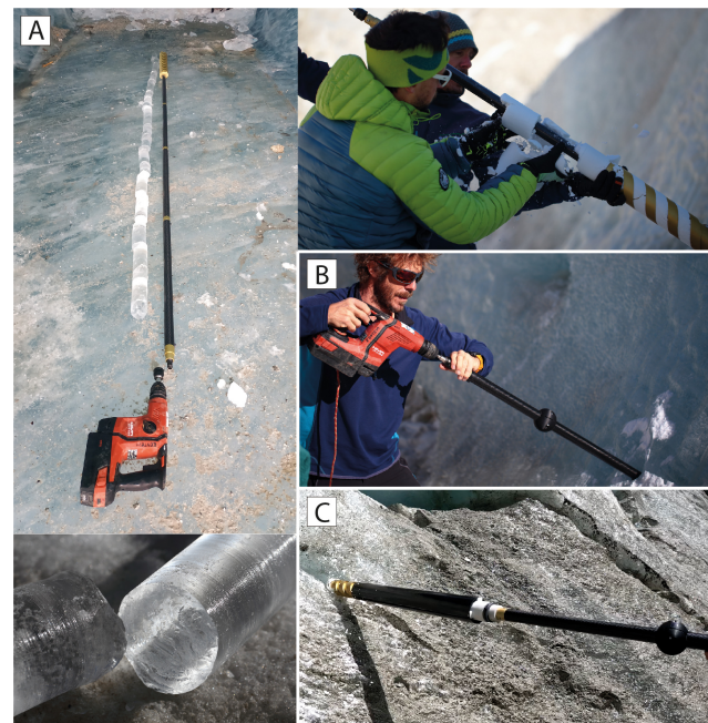
Figure 3. Coring tests carried out in October 2021 (A), June 2023 (B), and July 2023 (C). The first demonstrated the effectiveness of the drilling head but also the difficulties associated with the plugs formed by the ice chips. The second demonstrated the value of anti-vibration spheres fixed on the carbon extensions. The third showed the inefficiency of the chip chamber (black cylinder at the rear of the corer) and, one more time, the need to drill short sections of core to avoid ice plugs.
